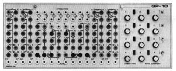
Summer-Integrators . . . Amplifiers 1 thru 4 may be used as summers, integrators, high gain operational amplifiers or as logic controlled, single pole, double throw electronic switches. Each has: a precision summing resistor network with patch panel gain 1 and 10 values; provisions for up to four integrating capacitors; a three mode electronic switch that is independently controlled with patch panel logic; an attenuator for entering initial conditions.
