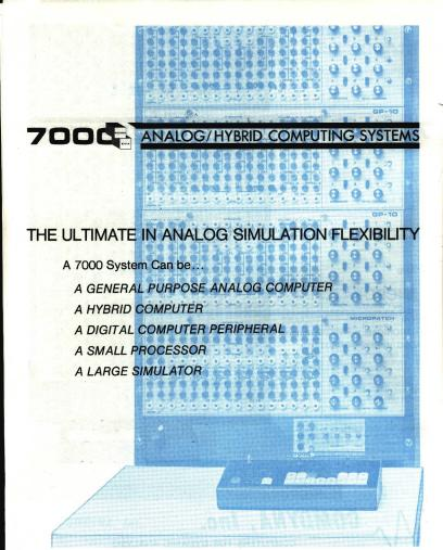
The 7000 Building Block Analog/Hybrid Computing Systems is an assemblage of analog computing units, accessories and interface networks that may be configured to meet small, medium or large simulation requirements.
